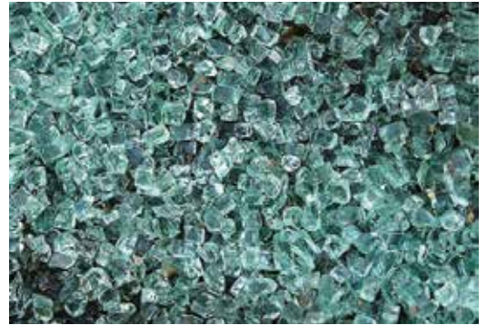
Broken Tempered Glass
